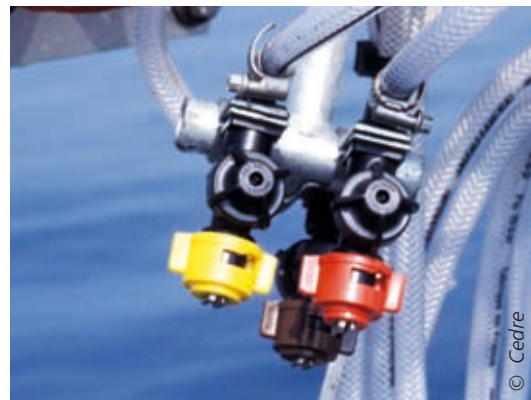
Nozzles fitted with check valves
