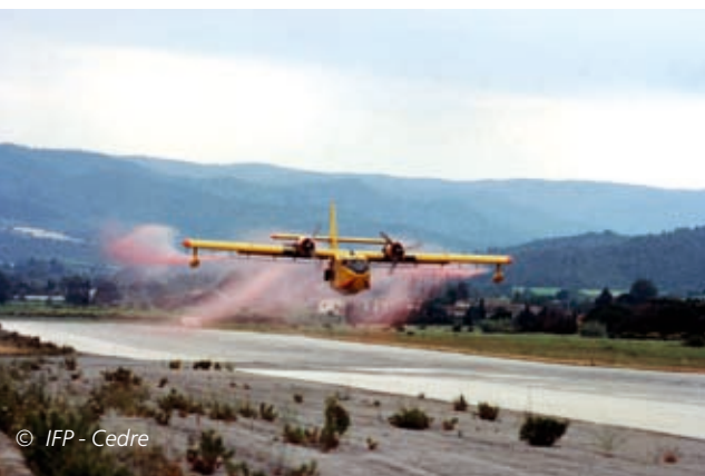
Calibration trials on the ground for dispersant spraying PROTECMAR trials
