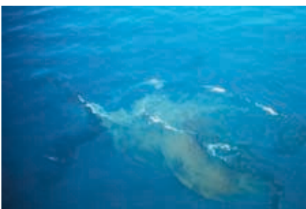
7, 8 - What the pilot sees: clouds of dispersed oil (beige) are quite distinct from the appearance of surface oil (which is black or metallic). Note on photo number 7 the presence of white foam which shows that they sprayed too much dispersant.
